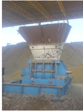
A factory hammer mill
